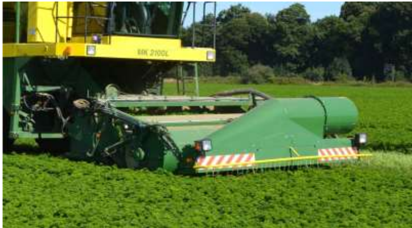
Ploeger MK 2100L plucking mechanism header with unique insect sucker blower attachment
